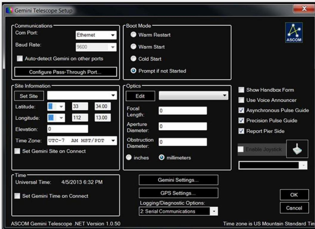
The above setup menu is what you will get if a Gemini-2 controller has not been detected. Notice you can still see Asynchronous Pulse Guide and Precision Pulse Guide. But if a Gemini-2 has been detected, you will get the menu below. Asynchronous Pulse Guide and Precision Pulse Guide are not shown. This is set because the Gemini.net driver sets them automatically with Gemini-2 systems.
