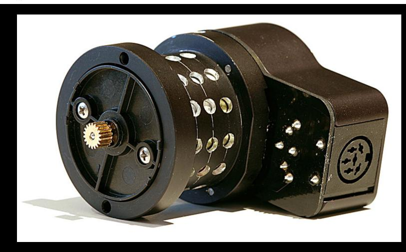
Complete motor unit after unscrewing off the gear box.
