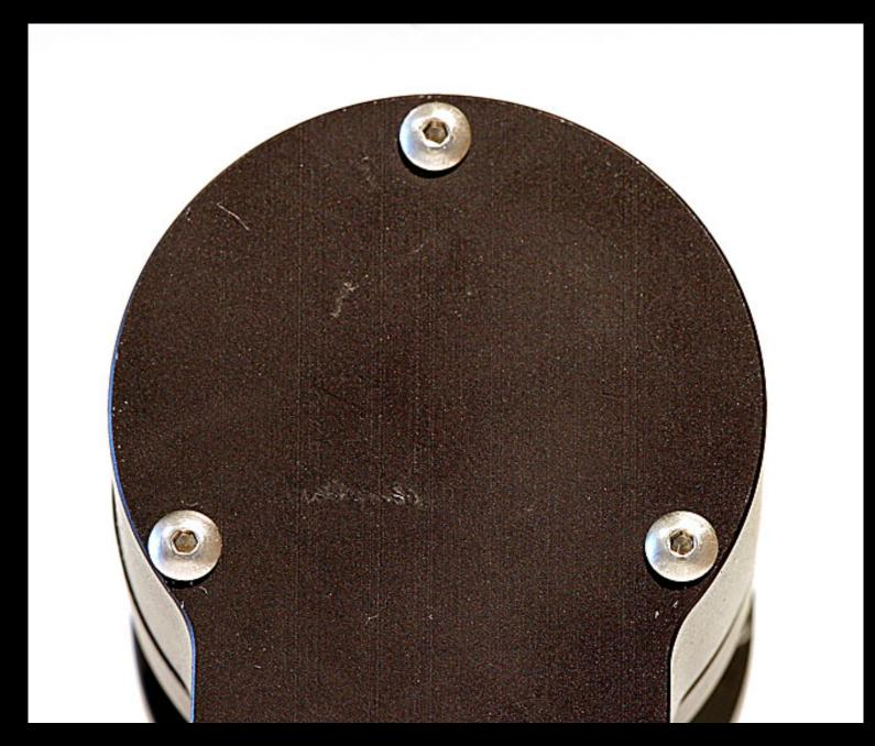
Unscrew this 3 screws and so the round cover of the motor slips from the motor click on image to next page
