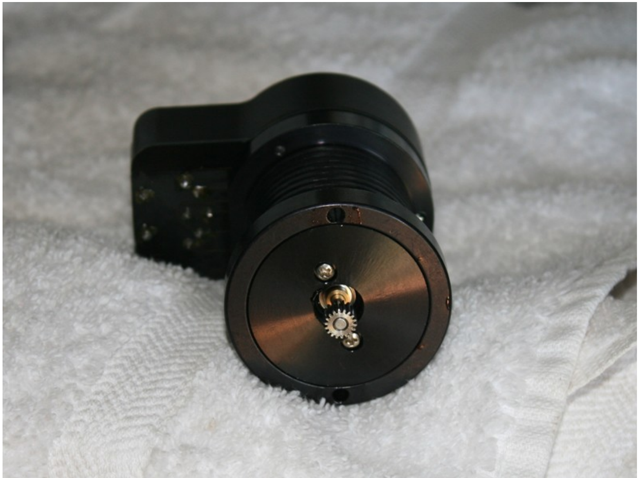
Figure 1. Maxon Motor from a Titan 50
