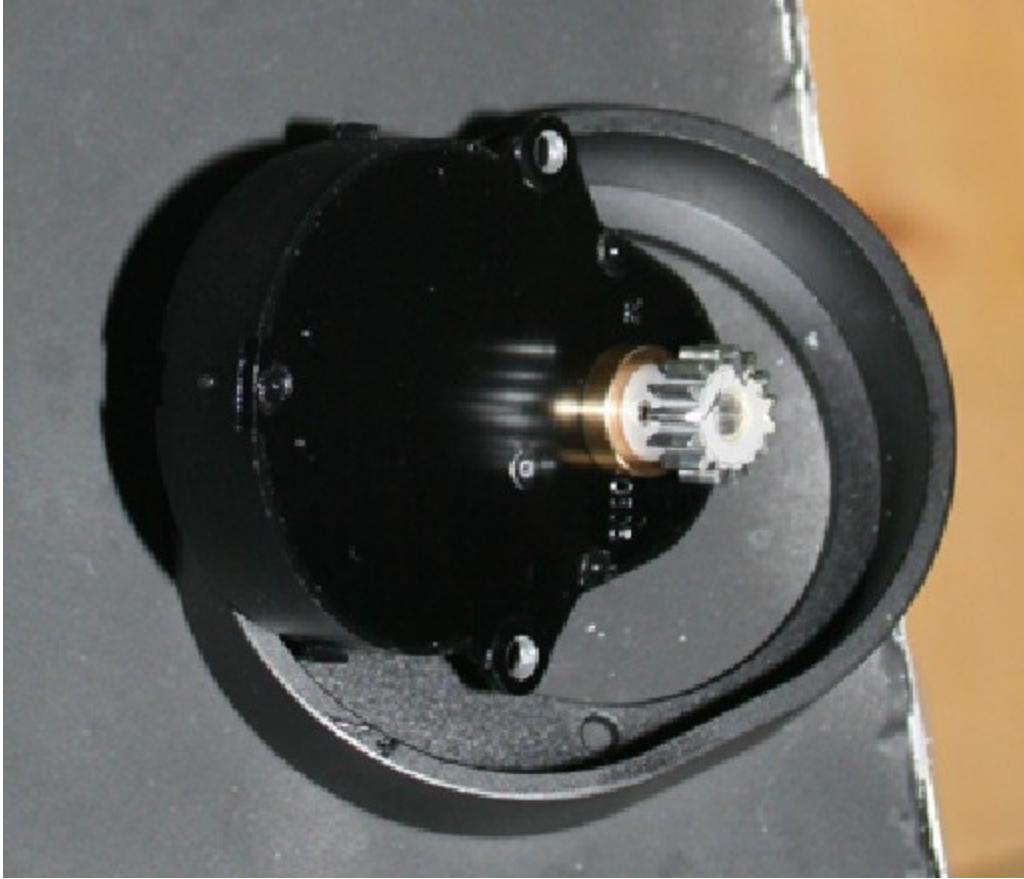
Figure 2. Spur Gear from a Titan 50
