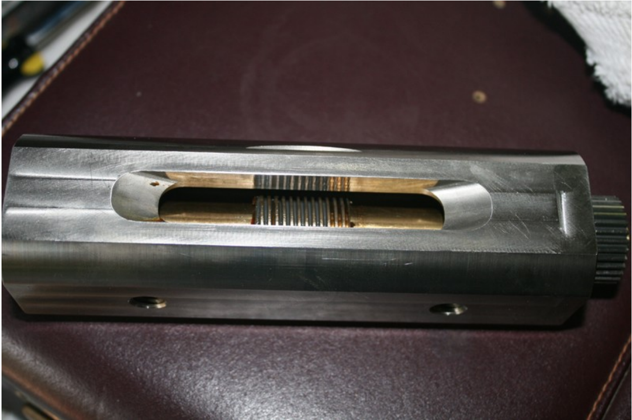
Figure 3. Worm Gear from a Titan 50
